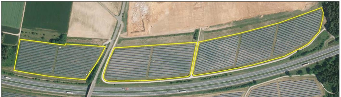
Figure 4: Example of a typical PVPP alongside a motorway. The PVPP consists of three plant areas (lds 44a-c). The total area (TA) and shape index (SI) vary between 2.08 ha/1.26, 2.31 ha/1.23 and 3.32 ha/1.40 (from left to right).
