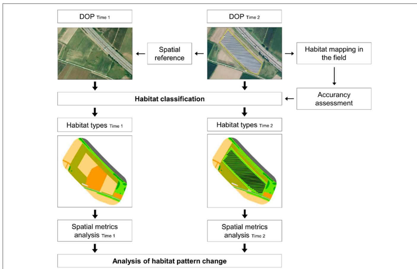
Figure 2: Technical flow chart (Data sources DOP: Image © GeoBasis-DE/BKG 2018)
