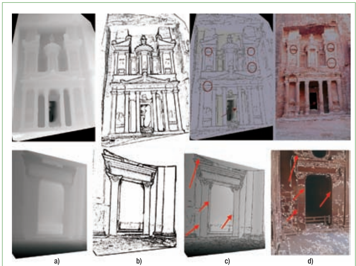
Fig. 6: a) Range images for 3D model of Al-Khasneh. b) Binary edge image produced using the proposed segmentation algorithm. c) Segmentation results after thinning process projected in the corresponding range image. d) Segmentation results of colored images using the proposed algorithm, the red arrows show some selected edges used for registration of 2D-3D data sets.
