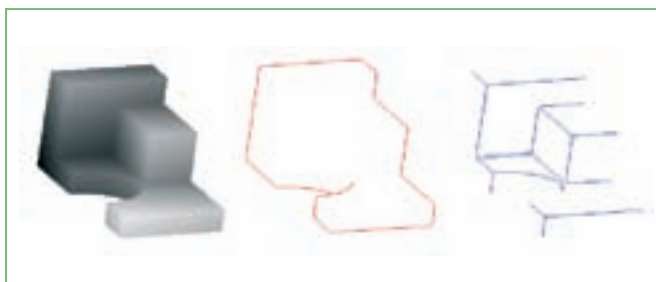
Fig. 5: Curve block segmentation using different thresholds to detect step edges (red) and crease edges (blue).
