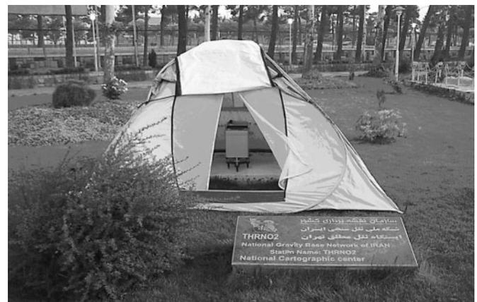
Fig. 2: Scintrex gravimeter at a gravity base station in Tehran
