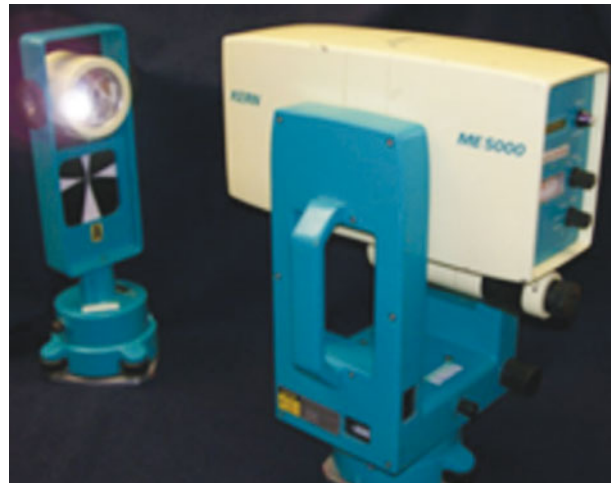
Abb. 1 | Mekometer ME5000 [ http://ppd.fnal.gov/align/images/mekometer.jpg ]
