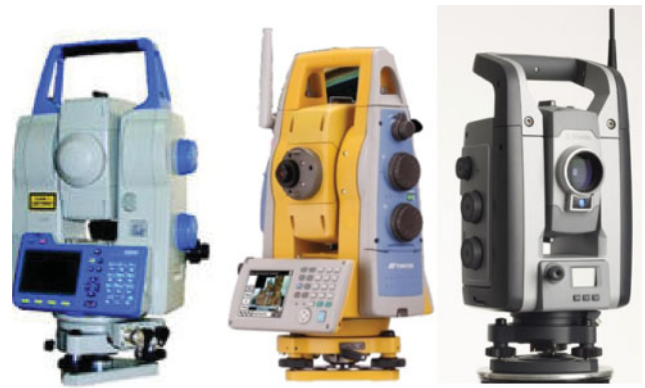
Abb. 1: Sokkia SET 3110MV – Topcon Imaging Station – Trimble VX Spatial Station
