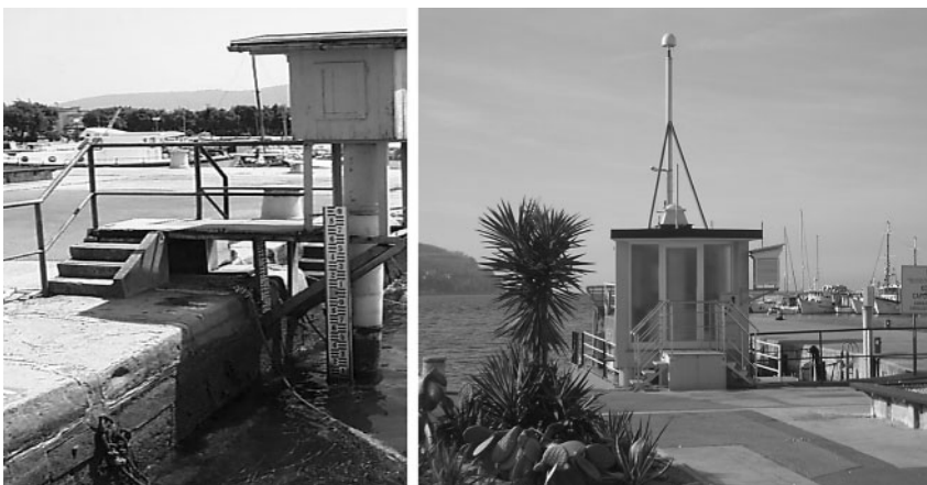
Fig. 1: The old tide gauge station of 1958 (left) and the new tide gauge station with the permanent GPS station (right)
