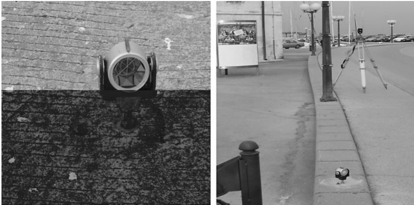
Fig. 4: Stabilisation and signalisation of reference points (left) and eccentric points (right) during the measurements
