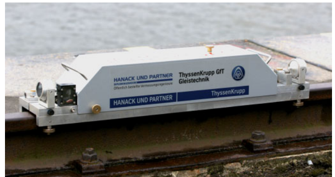
Figure 4: „RailControl“ monitoring vehicle.
