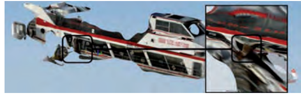
Figure 5 | Outcome of original “dock” image bundle. Rectangular shapes highlight errors caused by the triangulation
