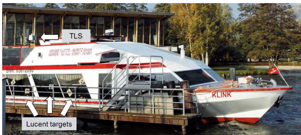
Figure 1 | Front part of the Klink with lucent targets prepared for image acquisition
