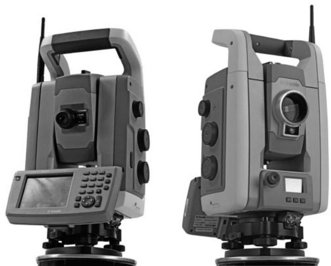
Abb. 1: Trimble S6 Totalstation
