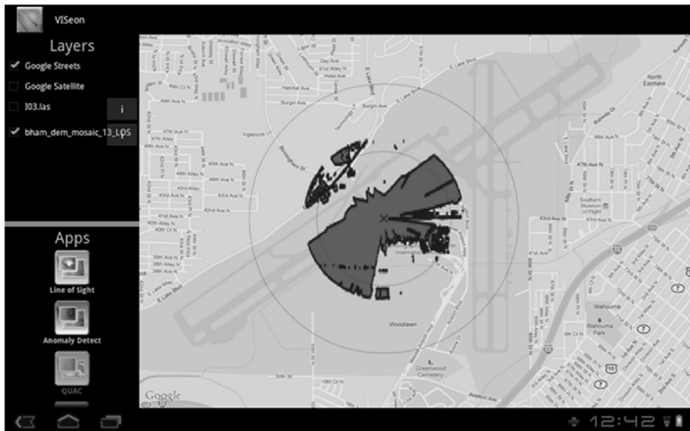
Fig. 3: An interactive Line-Of-Sight App, launched from Native Android Client. (a) The user locates an AOI, (b) draws an interactive circle to indicate parameters, (c) the middleware passes the location and AOI to the service, (d) the high-level service finds the appropriate data in the catalogue and constructs the ESE call, (e) the ESE runs and returns the vector result showing the line of sight, (f) the vector result is passed through the middleware to the client, (g) the client renders the result in the appropriate geographic location in the interface (EXELIS VISUAL INFORMATION SOLUTIONS 2012).
