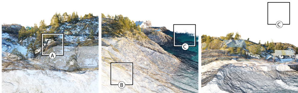
Fig. 6: Digital Pointillism , 2016: Point cloud generated via Structure from Motion (SfM) using Pix4D Mapper and UAV imagery, (A) Mixed point clusters, (B) Low point density / overly close, (C) Sparse or missing points / too far | Data processing: GRID-IT GmbH, Innsbruck | Drone Images & Visualization: Marc-Eduard Ihle
