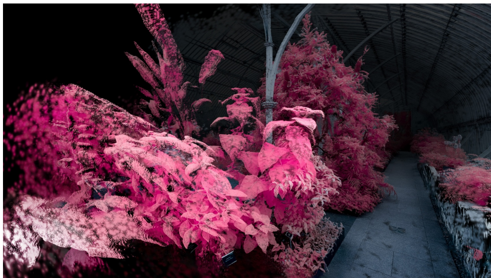
Fig. 5: SHARP-generated radiance field within a greenhouse at the National Botanic Gardens (Site 1). The lower-left region reveals the underlying 3D Gaussian splatting structure of SHARP within the foliage.
