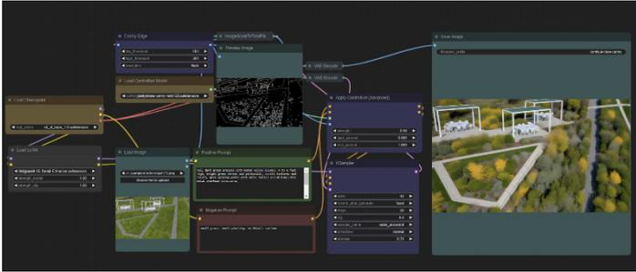
**Fig. 3:** ComfyUI node configuration displaying the base workflow with checkpoint and ControlNet Canny Edge integration for structural preservation in landscape architectural renderings
