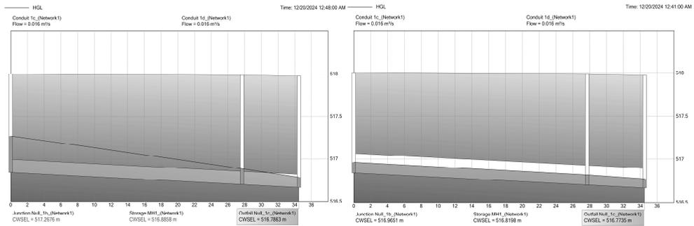
**Fig. 3:** Surcharging conditions produced under initial pipe diameter estimates in PCSWMM (left) and surcharging eliminated after pipe sizing was increased (right)
