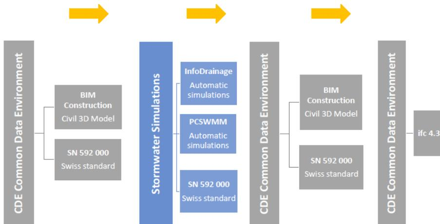
**Fig. 1:** Project workflow: BIM Site Engineering – Stormwater Simulations – BIM Site Engineering – ifc 4.3 (BIM Collaboration)
