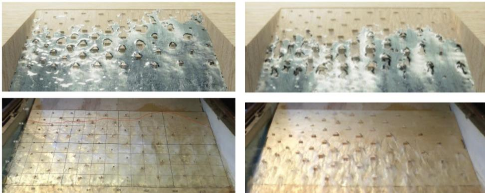
**Fig. 9:** Comparison of CFD simulations (top) and physical tests (bottom) for triangular texture. Left: comparison for up-flow. Right: comparison for down-flow.
