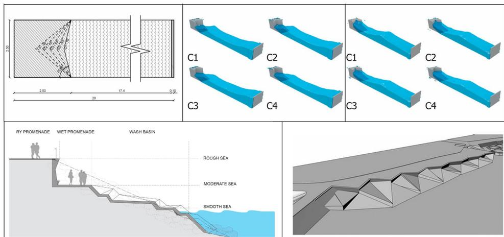
**Fig. 1:** Design for seaside promenade based on digital simulations of wave-seawall interaction under smooth, moderate and rough sea states (Source: GROBMAN 2017)
