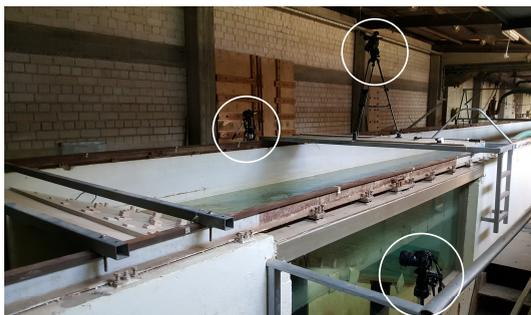
**Fig. 4:** CAMERI wave flume with three cameras marked with circles
