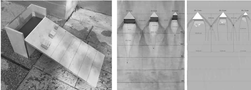
**Fig. 2:** Preliminary experiment. Left: mechanism for testing textured plates with constant down-flow. Middle: physical experiment. Right: CFD simulation.
