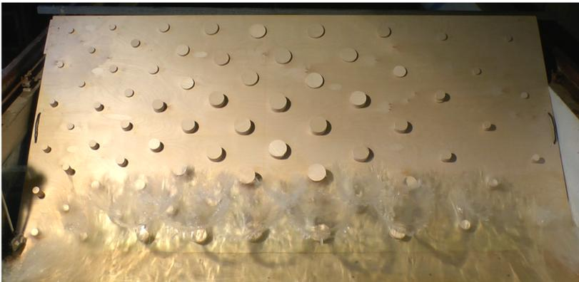
**Fig. 6:** Inverted trail created by upcoming wave for circular texture at 40 degrees slope
