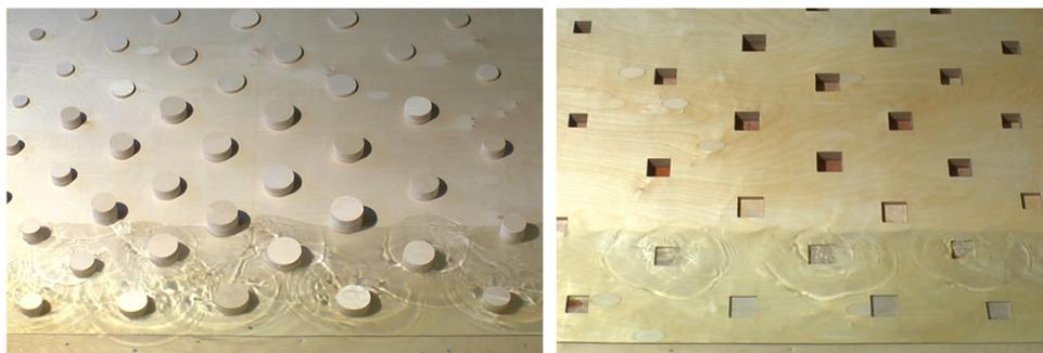
**Fig. 7:** Circular ‘echo’ traces created by upward flow of the first wave of the series
