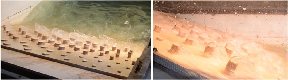
**Fig. 5:** Two views of the water jump created by returning wave for circular texture at 20 degrees slope
