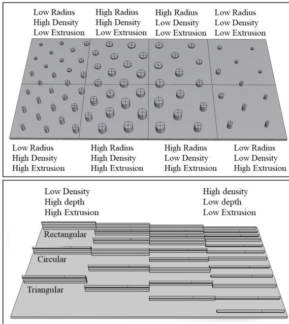
**Fig. 3:** Basic textured plates for second stage experiment. Top: Distribution of variations in density, extrusion and radius of point-based texture. Bottom: Distribution of variations in density, extrusion and geometry of line-based texture.
