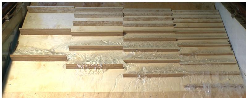
**Fig. 8:** Cascading effect by returning flow over a line-based texture plate
