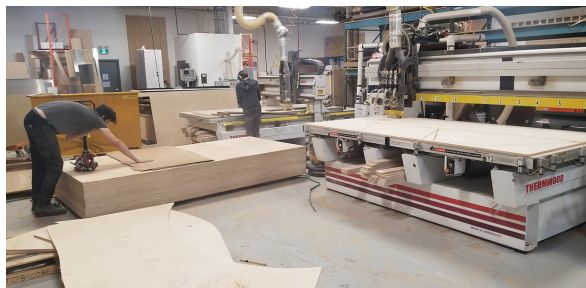
Fig. 10: The CNC machine cuts the wood panels based on provided construction documents
