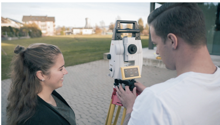
Fig. 9: The robotic station is central for stake out and site construction
