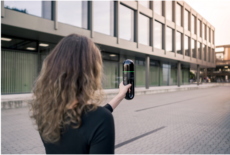
Fig. 10: Rapperswil students use handheld laser scanning devices as a regular tool for site surveying
