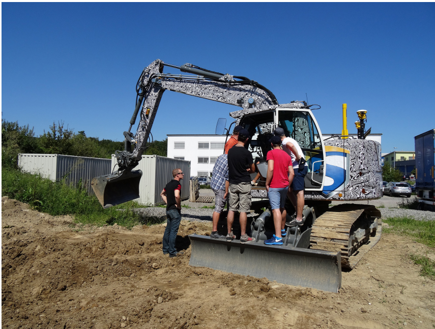
Fig. 11: Rapperswil students working with a 3D GNSS excavator on a construction site as part of the BIM2Field course
