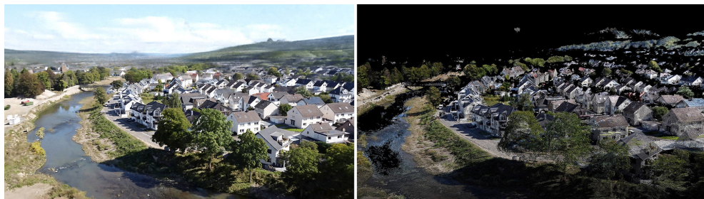
Fig. 5: Comparison of a NeRF model (left) and a model derived from photogrammetry (right) of the same area. The point cloud model is black in the background, while the NeRF model captures the depth of the landscape at several levels of resolution (NeRF model: SCHOB 2022; Drone imagery: REKITTKE 2022).
