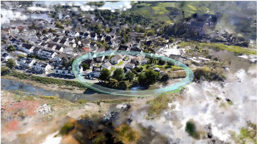
Fig. 4: NeRF model based on data extracted from a drone flight southwest of Ahrweiler, Germany. The frame circle in cyan shows the individual frames and the viewing direction of the drone flight (NeRF model: SCHOB 2022; Drone imagery: REKITTKE 2022).
