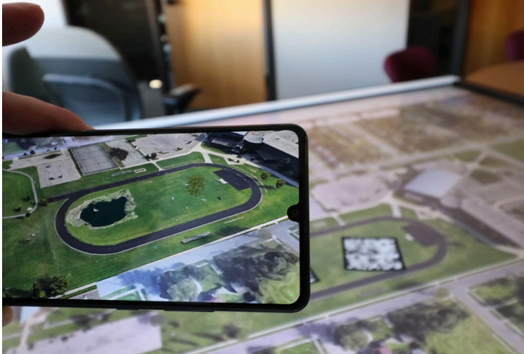
Fig. 3: Augmented reality version of Heilman Park on a touch table with the additional 3D models representing a tree and a pond provided by the paper targets
