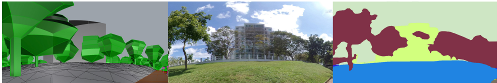
Fig. 8: An example whereby trees in the 3D model are opaque by nature (left) compared to those photographed on site (middle) and the image segmentation result (right)
