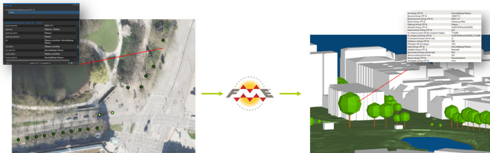
Fig. 4: Data transformation from 2D to 3D-IFC via FME. Left: 2D data from tree cadastre in Hamburg, with attributes of trees (pop-up window left). Right, after transformation: 3D trees as part of 3D city model, with identical attributes (pop-up window right) (BAREISS & GNÄDINGER 2022a).
