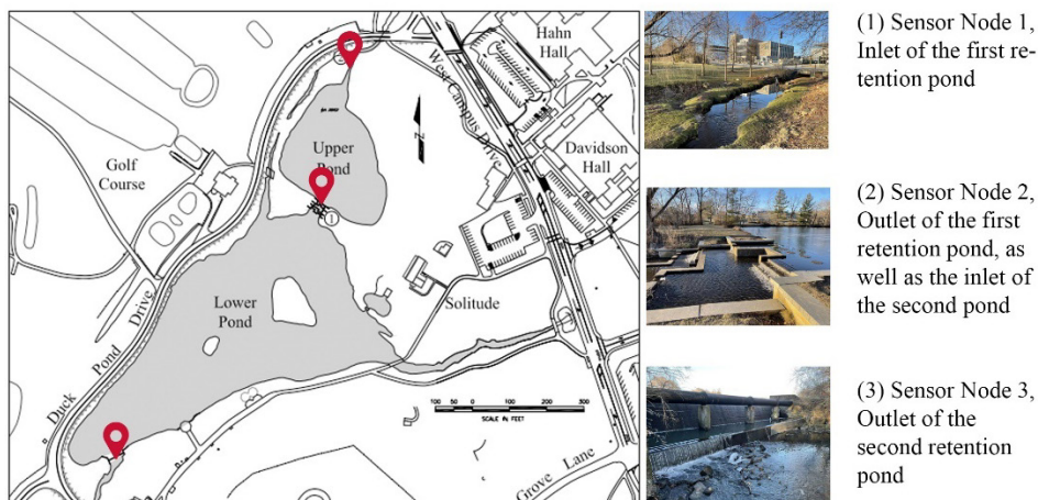
Fig. 2: This figure illustrates the experimental site, which includes two retention ponds, and presents the location of three sensor nodes
