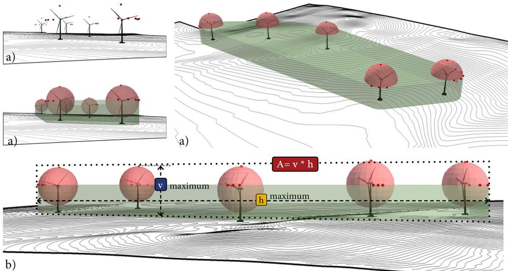
**Fig. 2:** a) Proposed wind farm bounding geometry defined by the location of turbines and potential multi-direction rotation of blades and modelling points; b) Measurable variables (v, h & A) to quantify DPVC using modelling points
