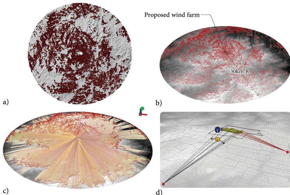
**Fig. 4:** DVC modelling: Observation points and sightline angles calculation in GIS; a) observer points identified within visible areas excluding treetops (plan view); b) perspective view of observation points in relation to the proposed wind farm within 30km radius surrounding landscape within ZVI; c) modelled 204,435 modelled sightlines for all observation points to the modelling points; d) Sightlines modelled for two sample viewpoints with different calculated variables
