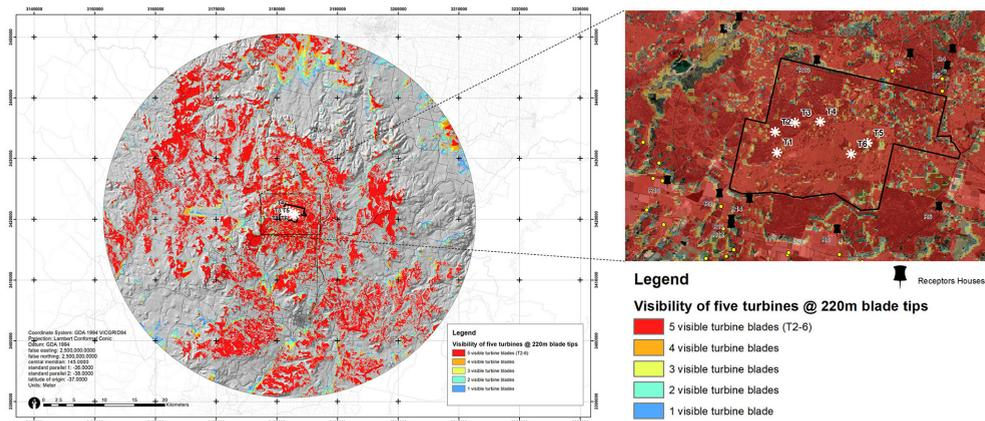
**Fig. 1:** Zone of Visual Influence (ZVI) of a proposed wind farm in Queensland including five turbines with 220m height to blade tips (2021)
