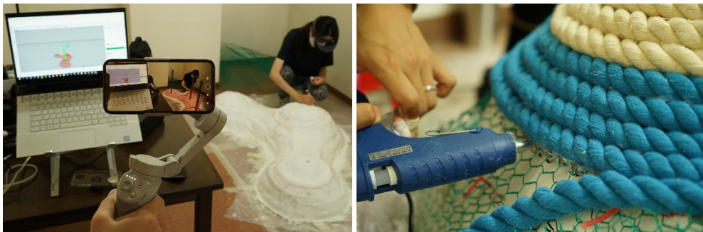
Fig. 4: Positioning rope with AR devices and winding with a glue gun
