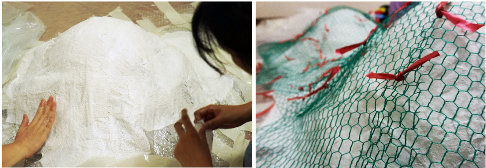
Fig. 3: Covering the object with plaster bandage and metal mesh wire
