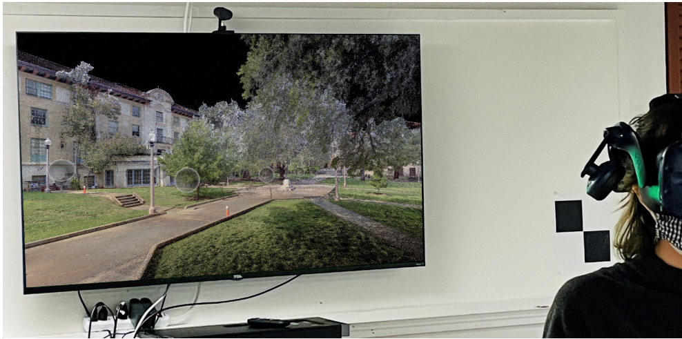
Fig. 3: Student navigating Unity3D Point Cloud model in VR
