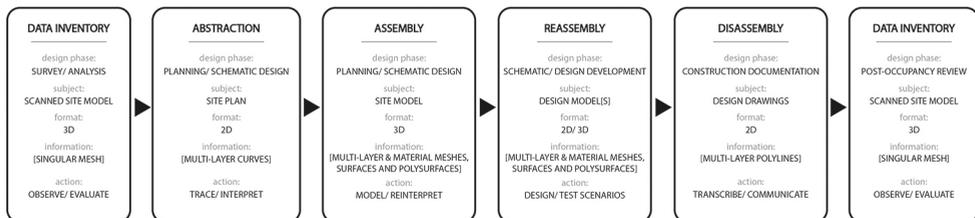
**Fig. 2:** Design process articulating the use of pre- and post-construction site scan mesh models within traditional landscape design practice workflow. Adapted from (URECH et al. 2020).
