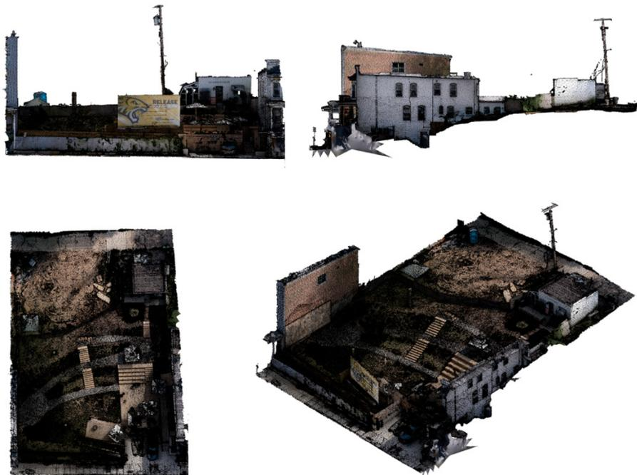
**Fig. 3:** Viewports (Front, Right, Top and NE Parallel Projection Axonometric) of post-construction site scan point cloud and mesh model in Rhinoceros 3D (1,029,881 vertices)
