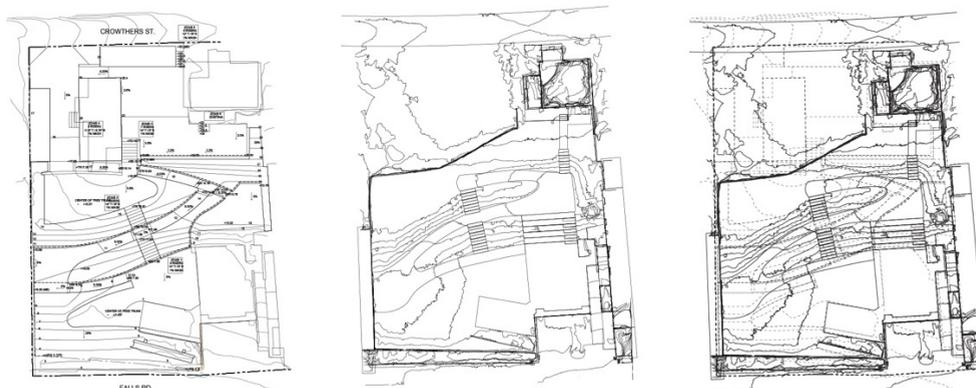
**Fig. 4:** 2D linework evaluating design proposal drawings in Construction Documentation phase (left) given to contractor, transcribed 2D linework from post-construction drone scan (center) and overlay of datasets (right)
