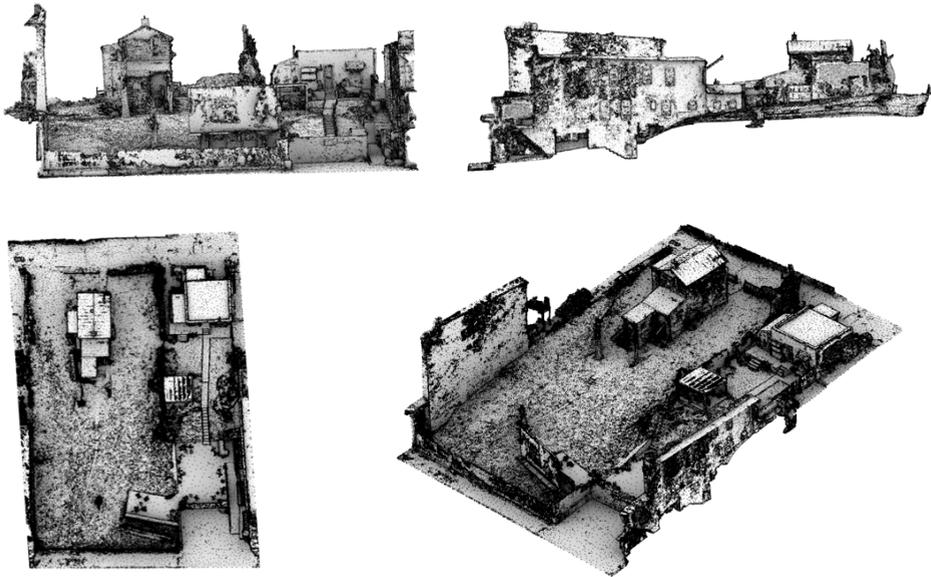
**Fig. 1:** Viewports (Front, Right, Top and NE Parallel Projection Axonometric) of pre-construction site scan point cloud and mesh model in Rhinoceros 3D (1,615,070 vertices)
