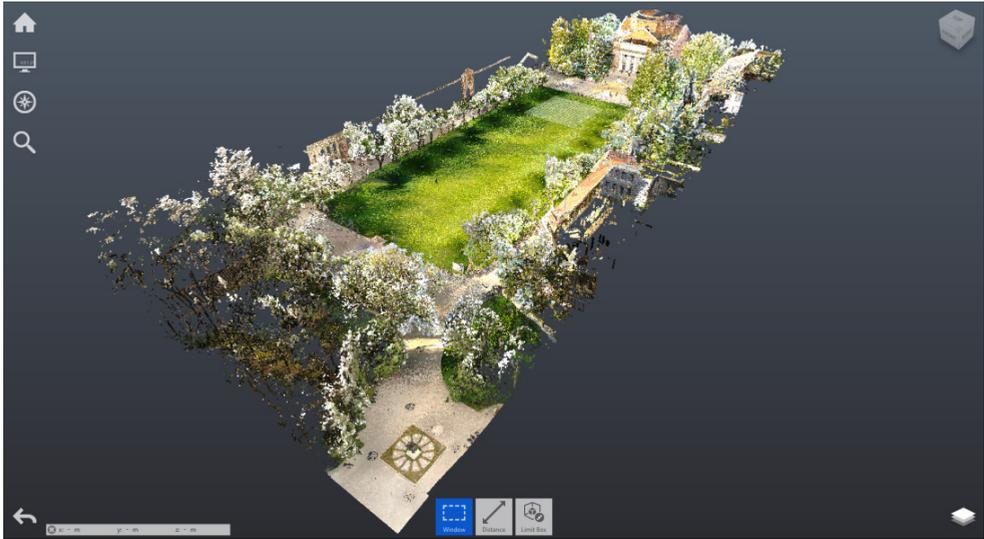
**Fig. 3:** Point cloud of the existing trees on campus deriving from TLS
