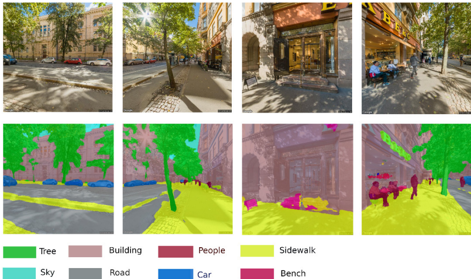
Fig. 3: Example of one datapoint representing a specific urban location. We use four street images of such a location which are then fed into an image segmentation method. The results of the segmentation are then used to construct the characteristic attributes (features) that characterize the datapoint (urban location).
