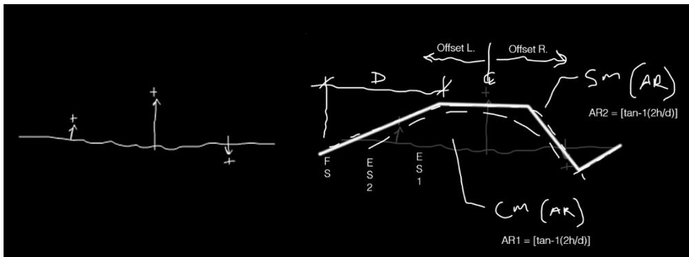
**Fig. 2:** With the “Centerline Curves” set to height the “Core Material (CM)” and “Shell Material (SM)” are deposited based on their respective specification and angle of repose
