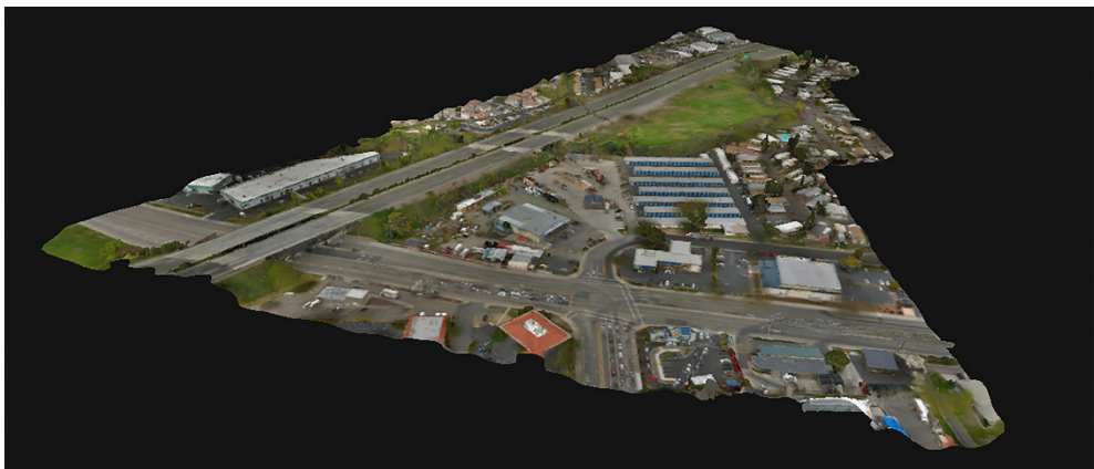
Fig. 2: Students conducted a virtual site visit using a 3D model developed with a point cloud and draped aerial imagery. Contextual oblique imagery, 360 panoramic images and on-the-ground photos complemented the model.
