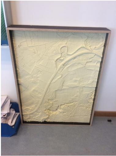
Fig. 1: The mould; an inverted DTM of the study area which was used to create the mock-up. Z -values were exaggerated 8 times
