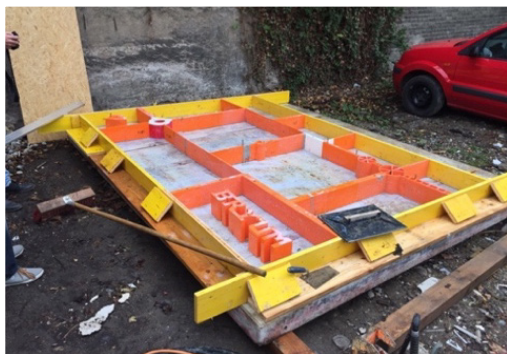
Fig. 5: Mold prototypes produced with the help of additive manufacturing processes (Source: WEINSBERG (2018, May 13), personal communication May 13, 2018, Image © BRYUM)
