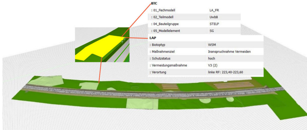
Fig. 4: Submodel UwbB in BIM coordination model
