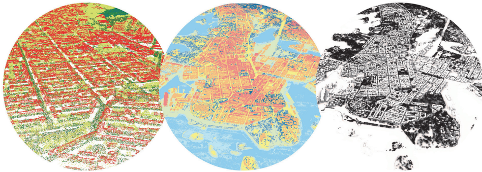
Fig. 1: The Helsinki LIDAR set in 2018 transformed to Digital Elevation Map and sky view factor for thermal simulation (Data from Helsinki Map Service 2017)
