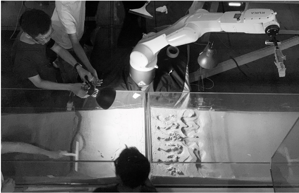
Fig. 2: Experimenting with the robotic feedback loop. Visible in the top-right is the tool holder on the robotic arm and perpendicularly attached to it the 3D scanner.
