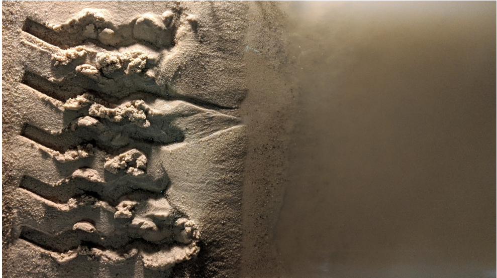
Fig. 6: Robotic sand formation after one manipulation cycle and a single simulated storm surge
