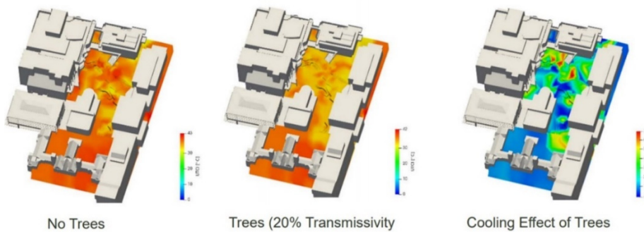
Fig. 4: The microclimate simulation model showing the impacts of a mature tree canopy coverage. Trees were shown to decrease the UTCI compensated temperature by up to 7 °C in hot conditions (AURECON 2018).
