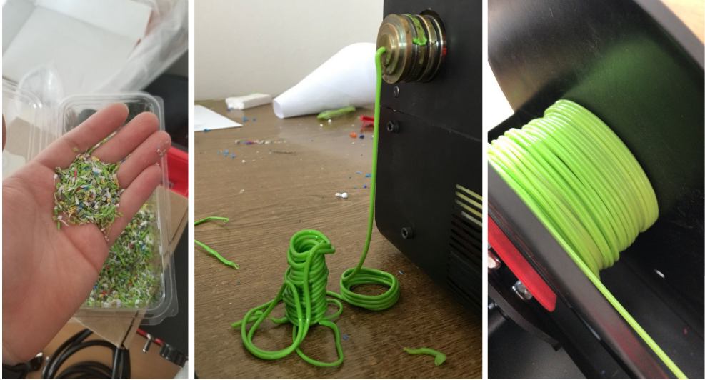
Fig. 3: Photos on plastic shredding, filament extrusion and spooling process
