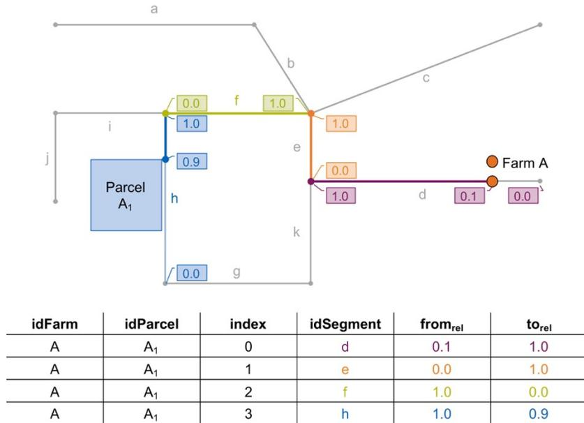
**Fig. 3:** Segmented representation of the farm-field transportation paths in the form of linear references to the elements of the road network
