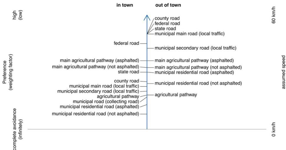
**Fig. 2:** Weighting factors and preferences for different road types are based on the assumed speed of a vehicle along a path segment
