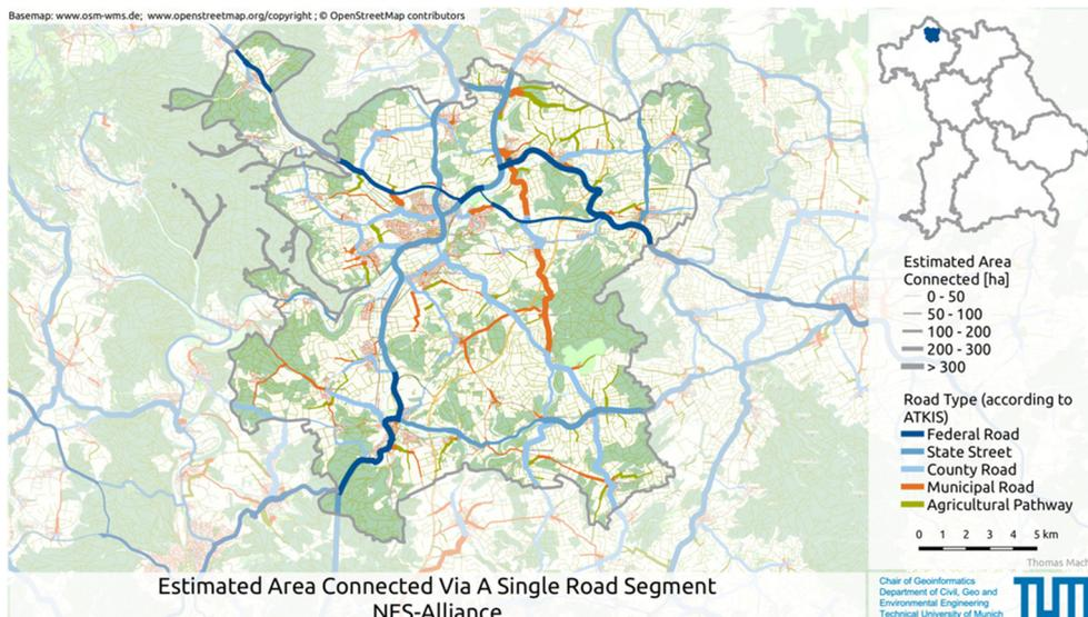
**Fig. 5:** Estimated area connected via a single road segment derived from farm-field transportation paths
