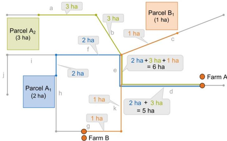
**Fig. 4:** Derivation of the indicator ‘connected area’ for road segments from single paths
