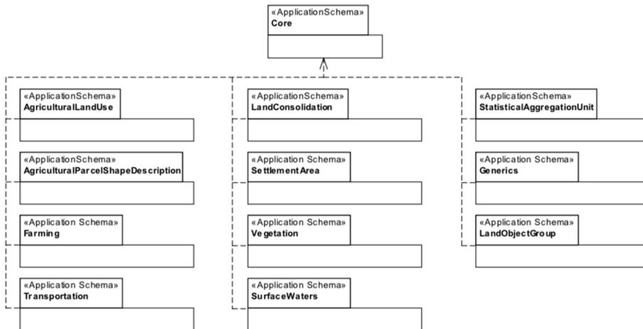
**Fig. 1:** UML package diagram of the aspects modeled in the information model of the LandModel<sup>TUM</sup>. Details on the data model are given in MACHL et al. (2015).
