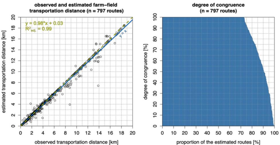
**Fig. 7:** Scatter plot of the observed and the estimated farm-field transportation distance (left); degree of congruence between the estimated and the observed transportation paths (right); data source: ASTNER (2017)
