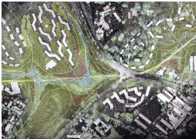
Fig. 3: The design modelled in three dimensions is projected in plan view and provides geographic information for height indications and contour lines
