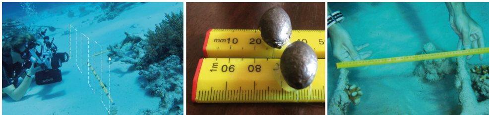
Fig. 6: ARP1-Setup (see Section 1.2). Taking photographs following lawn-mower pattern of one of the faces of ARP1, Portable plastic rulers with led attached were placed as reference next to ARP 1; about 200 manual measurements of ARP 1 were taken and documented.
