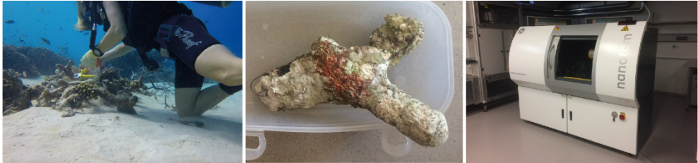
Fig. 9: From left: Extraction of sample; CT Scanner Nanotom M “research edition” at F.A. Finger-Institute for Materials Science of the Bauhaus-University Weimar
