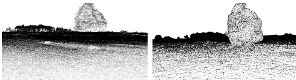
Fig. 1: Point cloud representation (left) and mesh-based representation (right) in black and white graphics that highlights the difference between geometries. Point clouds are simple discrete points that can be seen through, whereas mesh is a surface.
