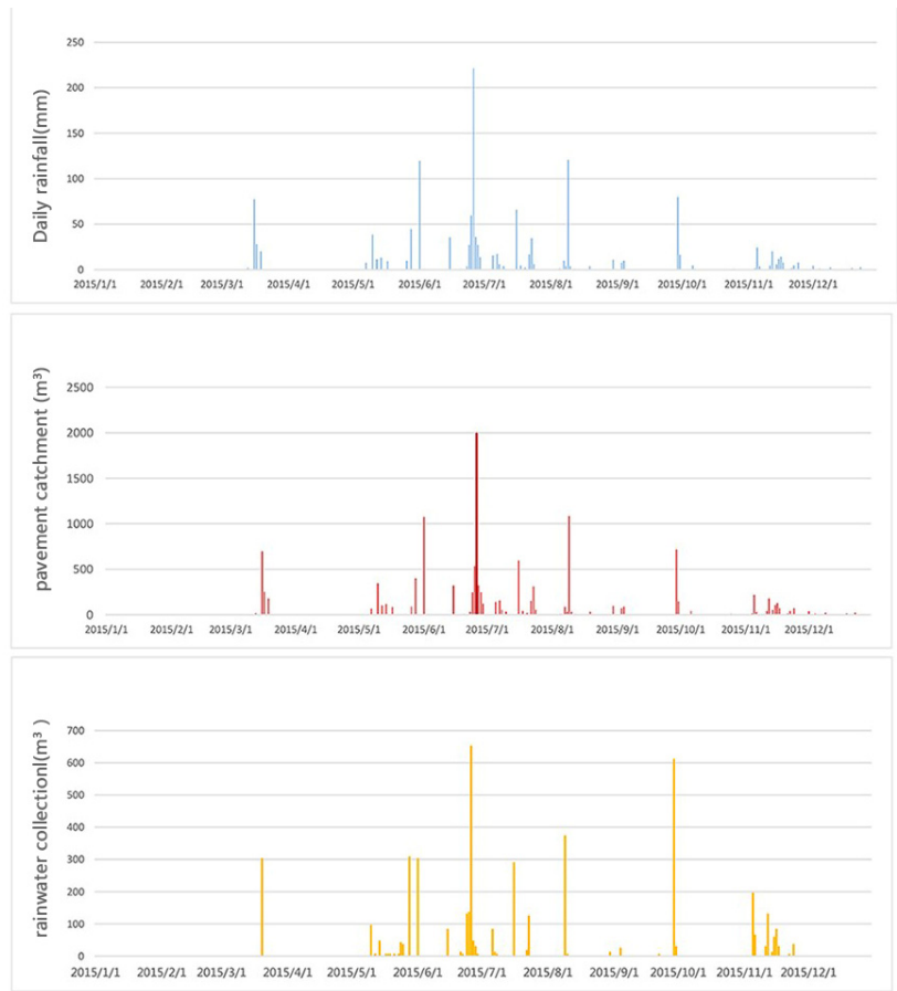
Fig. 5: Statistics of site daily rainfall, pavement catchment and rainwater collection from July 2016 to July 2017 in Nanjing Tianbao Street eco-road
