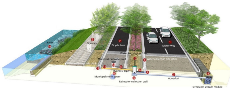
Fig. 1: Eco-road system diagram of Nanjing Tianbao Street
