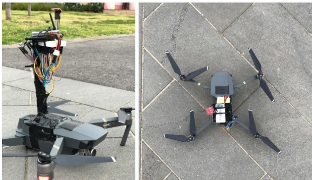
Fig. 1: Environmental sensors propped by a 3D printed stand attached to the DJI Mavic aircraft
