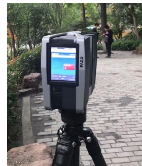
Fig. 4: FARO330 3D laser scanner
