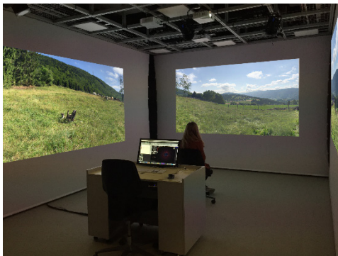
Fig. 1: Setup of the experiment in the AudioVisual Lab: The participant in the middle of the room is looking at the panoramic projection of a landscape type and hearing an ambient sound prepared for this scene
