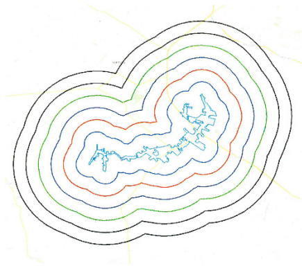
Fig. 4: Buffer distances around settled areas are used to identify sections of the horizon which are covered by wind farms
