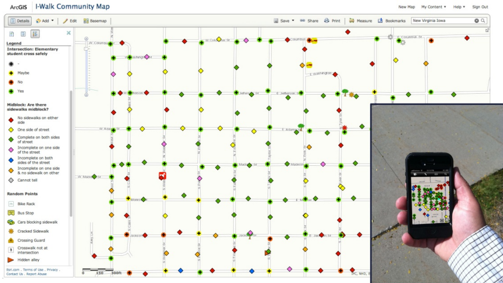
Fig. 3: During the data collection workshop the display of collected data on a device and on ArcGIS.com identifies where data still needed to be collected and the status of the infrastructure at the collected location. Following the workshop, this information is overlaid and analyzed with traffic accident data, locations identified in the geospatial user survey as perceived risks, and other mapped data.
