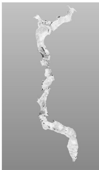
Fig. 4: Result of the registration – view from the top of the 3D model of the Eisriesenwelt (FARO Scene Version 4.8.2.)
