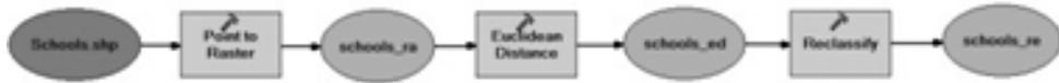
Fig. 3: First workflow segment from the raster conversion, to the Euclidean distance calculation, and finally to the reclassify process.
