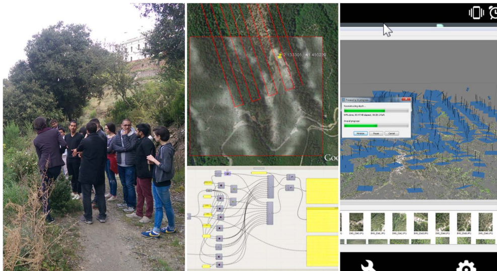
Fig. 2: While on an extended site visit (left) the on-site generation of UAV flight paths, generated from Grasshopper script and exported to the UAV, (centre) to generate the required data in the hills above Barcelona, Spain, (right), being processed remotely for additional speed and data fidelity (ETHZ/IAAC)
