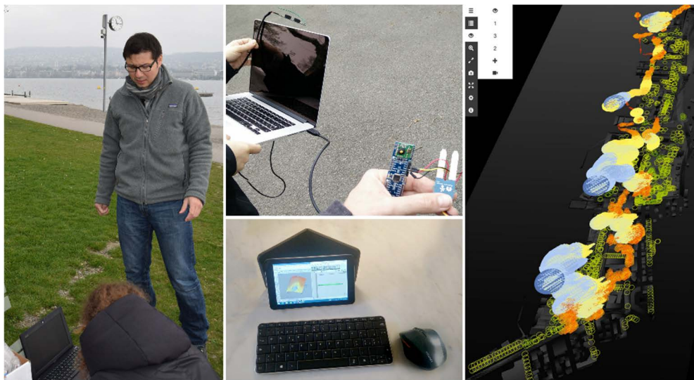
Fig. 4: Sensor deployment (l), on-site landscape analysis on laptop & tablets (m), used in aiding the optimal placement of soil moisture sensors. Resulting in local terrain visualisations (r) combining open space network analysis and microclimate data.
